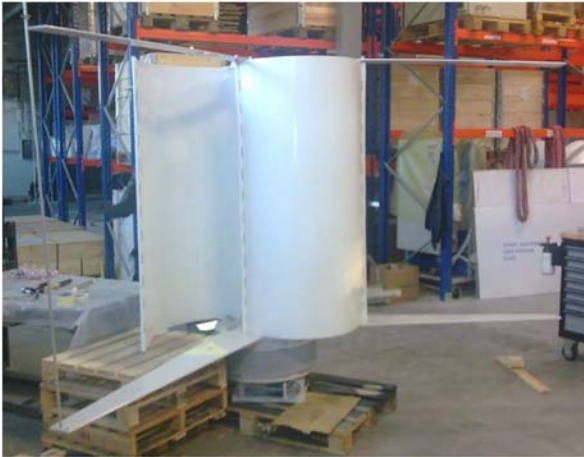
Fig. 8.4. Generator with half-assembled H-type wind turbine (with Savonius).
