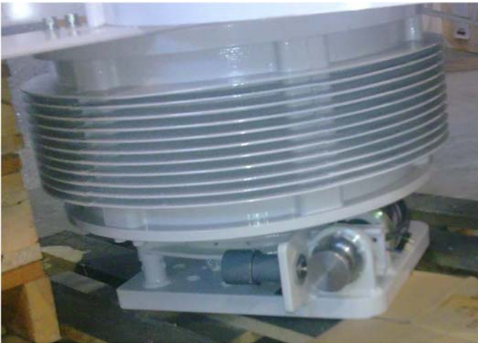
Fig. 8.3. A photo of the 5 kVA permanent magnet generator with outer rotor.
