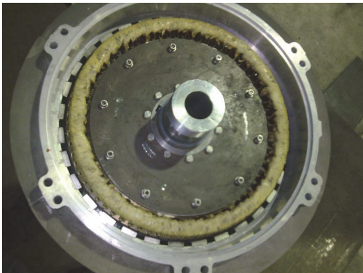
Fig. 14. A photo of the 5 kW permanent magnet generator with outer rotor.
