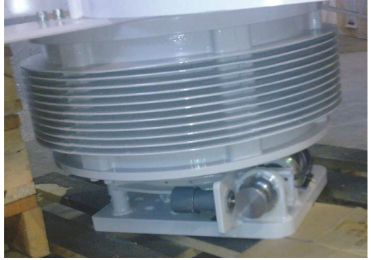
Fig. 15. Assembled PM generator.
