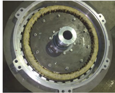
Fig. 9. Prototype generator with outer rotor.
