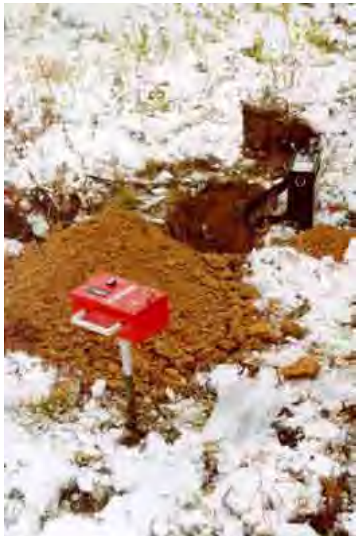
Figure 4. Measurement of radon in soil air with MARKUS-10.
