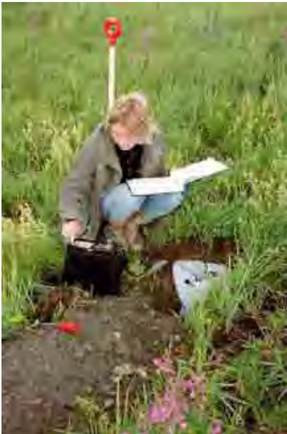
Figure 3. Margit Enel performing a gamma spectrometer measurement. The detector unit is located in the plastic bag in the hole.
