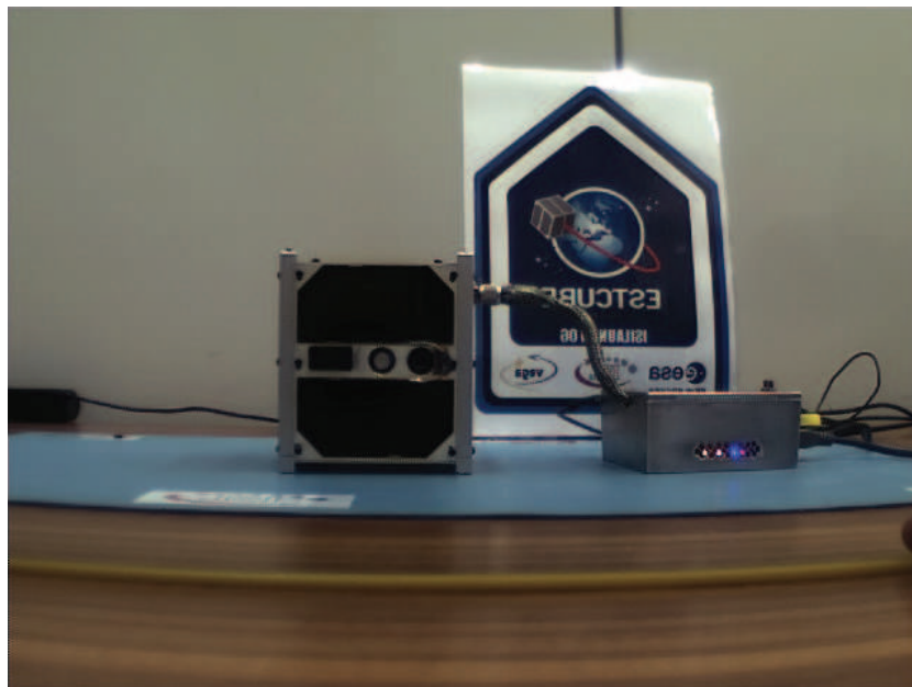
Fig. 8. A photo of the satellite in the mirror, made by the camera onboard the satellite at the Guiana Space Centre in Kourou. The satellite is connected to the access port device, which is used to communicate with the satellite before launch.
