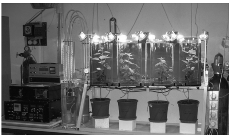
Fig. 1 Photograph of the computer-controlled growth chamber and gas exchange system used to control the ambient [\text{CO}_2] during canopy development.
