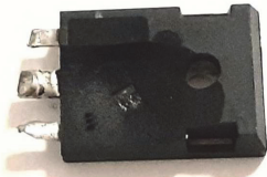
Fig. 3: Example of case damage to a SiC MOSFET featuring OCF.
