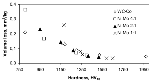
Fig.8. Volume loss vs. bulk hardness of the tested carbide grades
