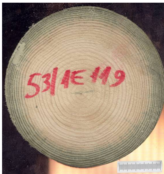
Fig. 4. Results of impregnation tests of pine roundwood with Tanalith-E agent
