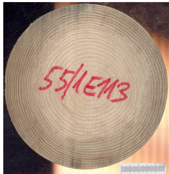
Fig. 5. Results of impregnation tests of pine roundwood with Rape-seed oil based emulsion
