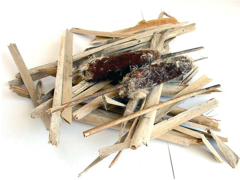
Joonis 1. Hundinuia kütus: W^t = 30\text{--}40\% , Q_a^t = 9\text{--}10 \text{ MJ/kg} , E^t = 2,5\text{--}3,0 \text{ MW}\cdot\text{h/t} , A^k = 5\text{--}6\% Figure 1. Cattail fuel: W^r = 30\text{--}40\% , Q_i^r = 9\text{--}10 \text{ MJ/kg} , E^r = 2.5\text{--}3.0 \text{ MW}\cdot\text{h/t} , A^d = 5\text{--}6\%
