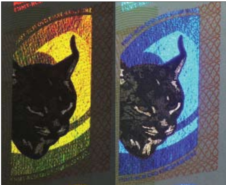
DOVD – kinegramm valguse langedes erinevate nurkade all.
