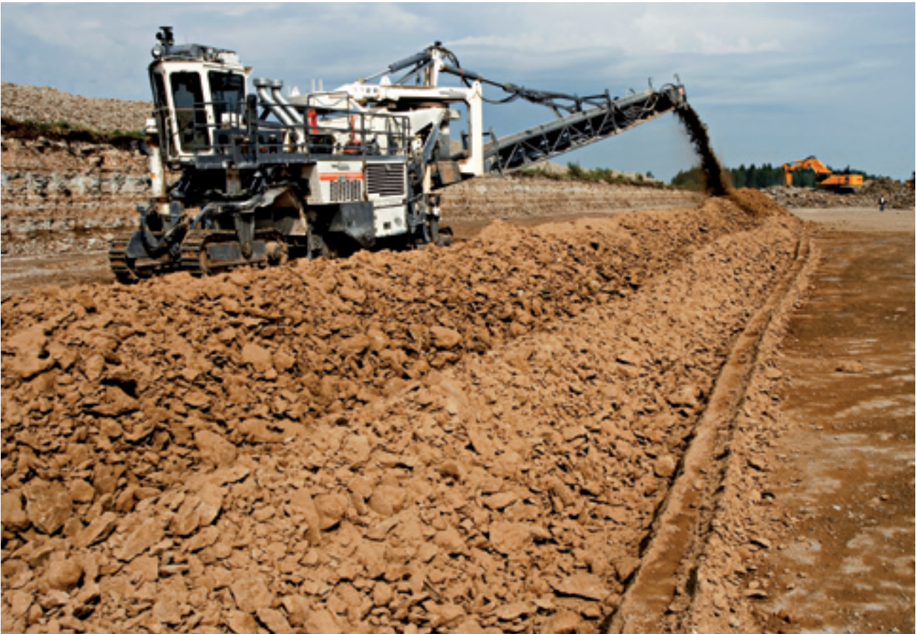
Oil shale mining in the Põhja-Kiviõli open-cast mine: mining of D-F 1 oil shale sequence (above). Surface miner Wirtgen 2500 SM allows selective mining of individual oil shale beds as well as limestone interbeds.
