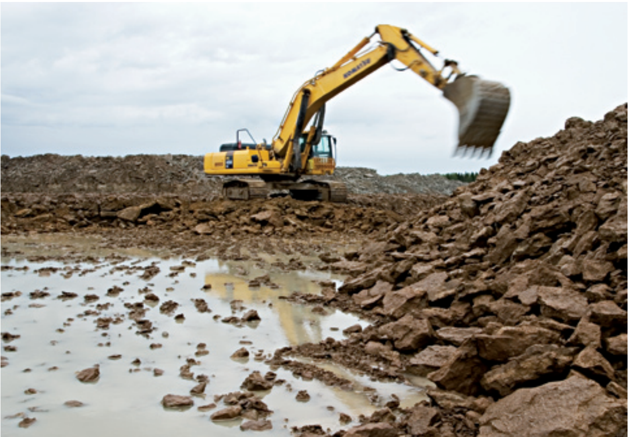
Oil shale mining in the Põhja-Kiviõli open-cast mine: mining of D-F 1 oil shale sequence (above). Surface miner Wirtgen 2500 SM allows selective mining of individual oil shale beds as well as limestone interbeds.
