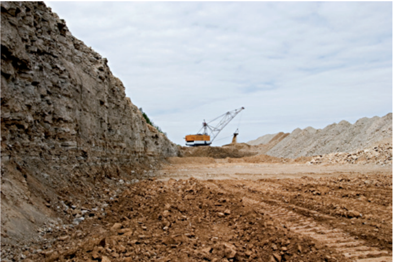
Dragline removing overburden
