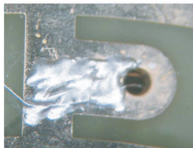
Fig. 8. Slip ring bond. (a) Basewire and three gold wires bonded on the slip ring. (b) Closeup of the same bonds. (c) All bonds covered with conducting glue.
