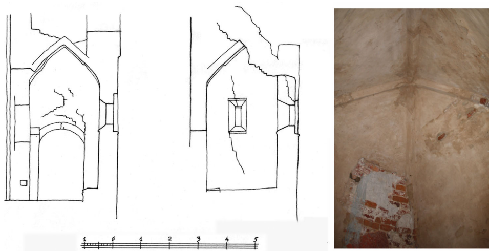
Fig. 3. St Nicholas church at Lipno near Novgorod (1292). Covered vaults in the corner chambers of the catechumena. Draft by Petr Maksimov (Maksimov 1952, 97). Photo by Ilya Antipov.
