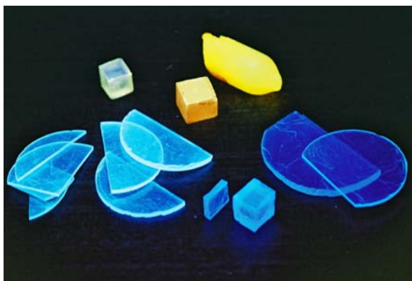
Fig. 1. Main investigation objects at the Institute of Physics of the University of Tartu: luminescent crystals, grown at the Institute.
