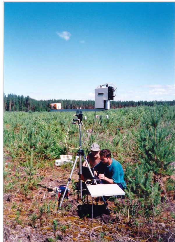
Field measurements by a GER-2600 spectrometer in a young stand at Konguta. Dr A. Kuusk and doctoral student M. Lang calibrating the spectrometer by a reference panel.
