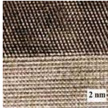
Fig. 2. An Al 2 O 3 (top) – SnO 2 (beneath) junction, as displayed with atomic resolution with the aid of a tunnel microscope.
