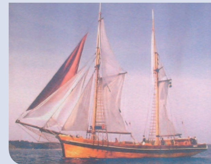
Hoppet av Spithamn. Length: 21,82 m, breadth: 6,84m, draught: 2,1m, weight: appr. 60 tons, including 15 tons of lead ballast.
